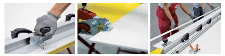
• When planning a cut that will be the full length of the panel, either with a plunge cut, or starting at the edge, mark and drill a relief hole at the termination point of the cut, then cut towards the relief hole. Properly support piece equally across entire surface of the piece when setting in mortar and prior to handling for installation.
